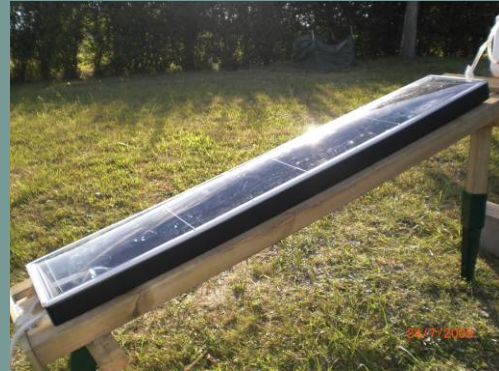
Type: SolarDew One Location: South West France Capacity: 7-12.5 l/day Year of installation: 2009 Still in operation: yes Usage: drinking water production
