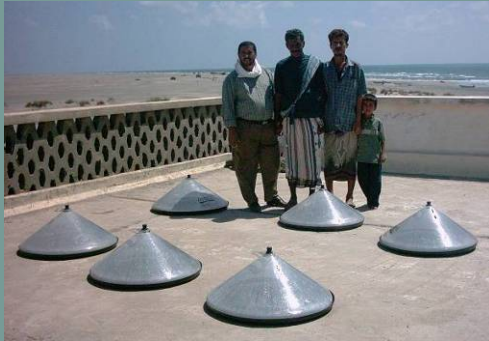
Type: solar still Location: Yemen Capacity: 1.5 l/d Year of installation: 2007 Still in operation: yes
