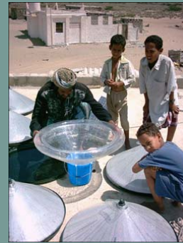
Type: solar still Location: Yemen Capacity: 1.5 l/d Year of installation: 2007 Still in operation: yes
