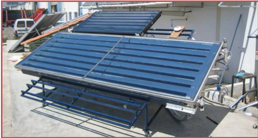
MAXI (5.5m 2 area) and AO SOL's standard product CPC 3E (2m 2 area). Being tested in AO SOL's factory test bench.
